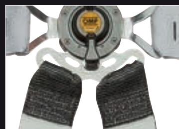
Exclusive double pin T-bar crotch attachment.
