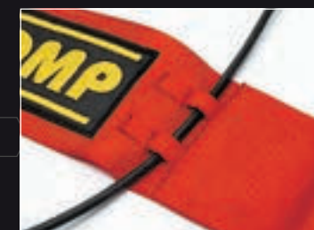
Runner for fixing intercom connectors.
